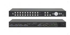
VP-732 is a 10-input presentation switcher/dual scaler with four HDMI, two DisplayPort and four user-definable (universal) analog video inputs. It upand down-scales to selectable graphics or HDTV output resolutions to preview and program outputs (up to 4K30 UHD on the program output) and provides ultra-fast fade-thru-black switching between sources. VP-732 supports analog and embedded audio inputs and outputs and includes rich audio functionality and a stereo loudspeaker output
